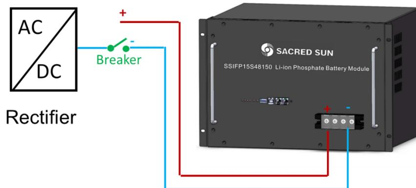
Figure 5-2: Single Battery Connection
