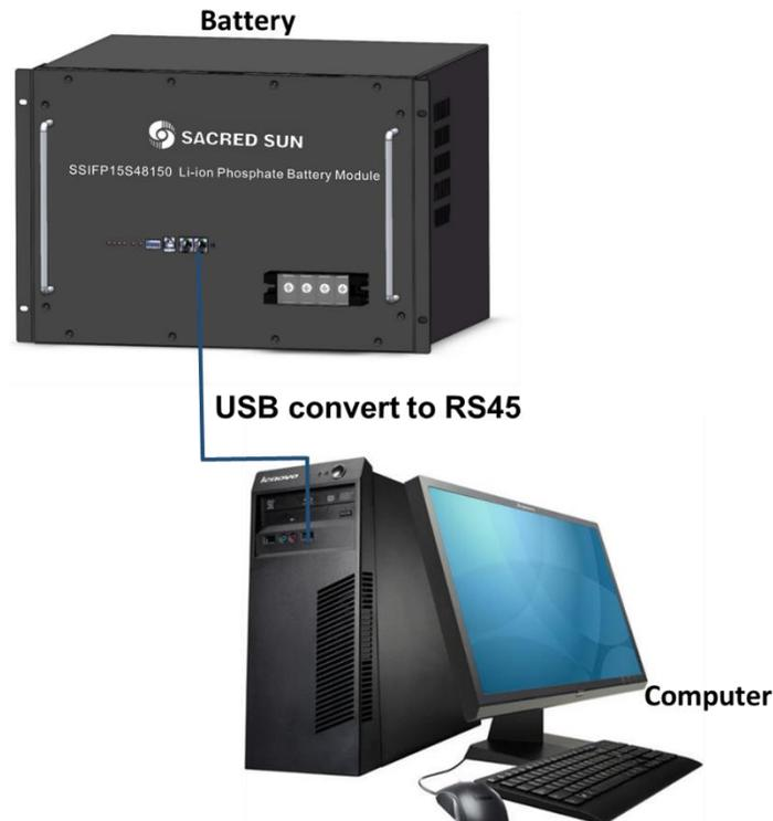
Figure 5-3: Communication Cable Connections between Battery and Computer
