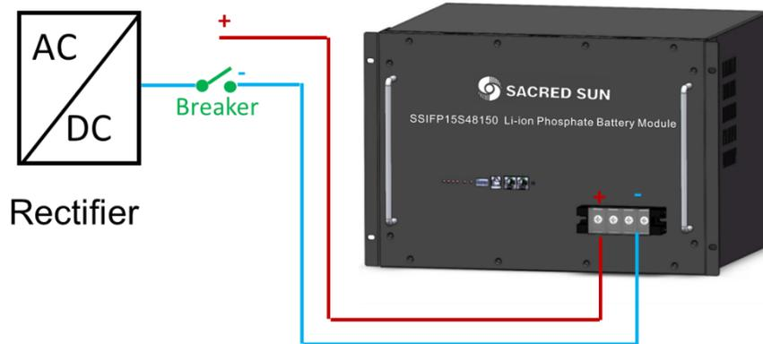
Figure 5-2: Single Battery Connection
