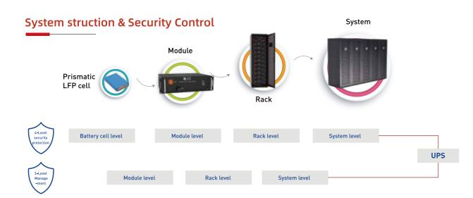
Three-layer BMS system ensures the reliability of lithium batteries layer by layer.
